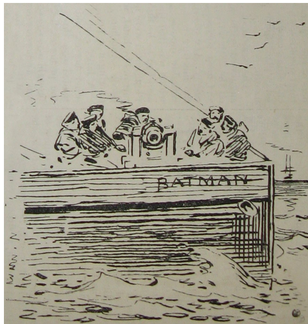
Figure 51 - Batman with its Temporary 64 pounder Bow Gun.
