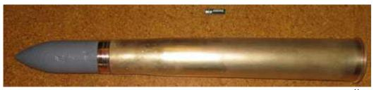
14 pdr projectile (in undercoat grey) and shell casing (800 mm) with AA battery for scale. 11
