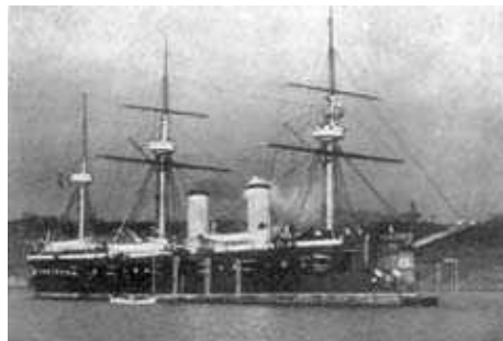
Russian Turret Cruiser Dimitri Donskoi four 8-inch breech-loading guns, twelve 6-inch breech-loading guns waterline belt of 6-inch compound armour
